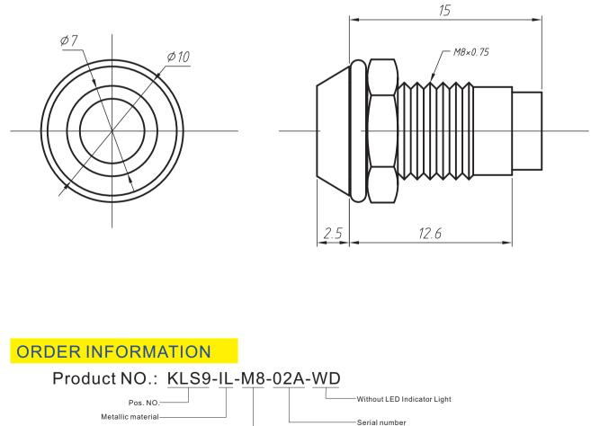
Metallic material Mounting Hole:  $\Phi$  8mm
